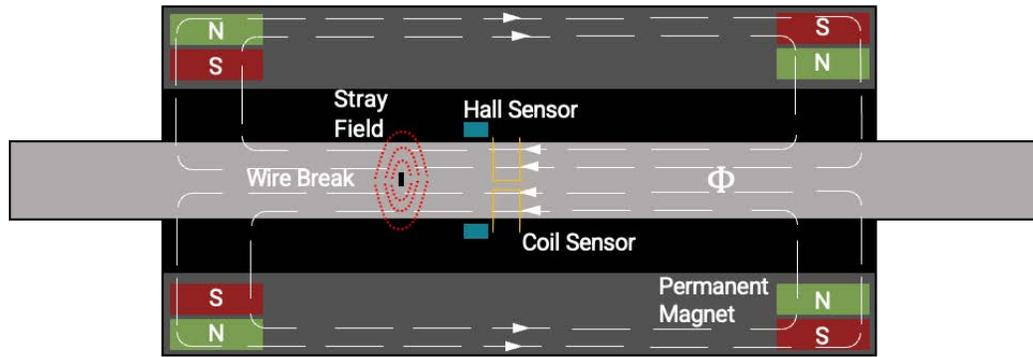
Figure 3. Principal setup of a MRT device.
