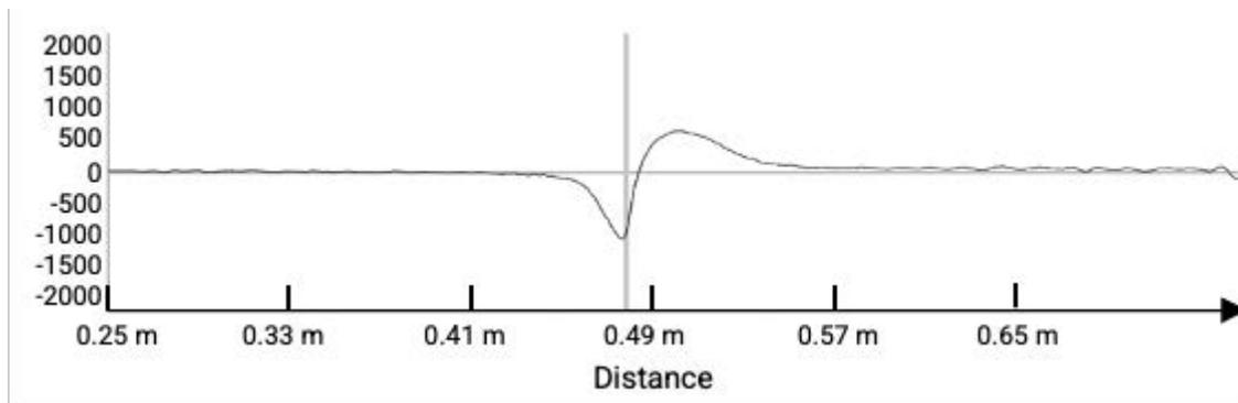
Figure 4. Characteristic magnetic flux leakage signature from a coil signal, with the shape representing the defect.
