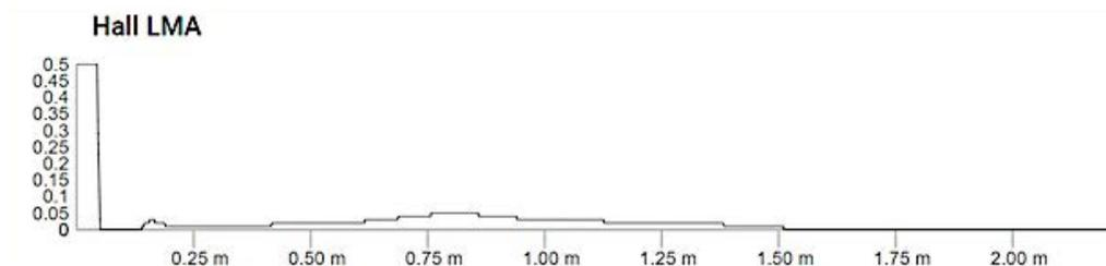
Figure 6. Hall-LMA Signal showing cross-section reduction in percentage.
