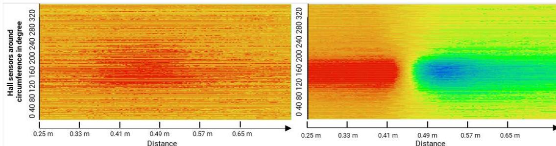
Figure 5. Heatmap generated from Hall effect sensors for defect located in the cable center of a 127-strand cable, magnetization in the center 1.425 T (left), magnetization in the center 1.9 T (right).
