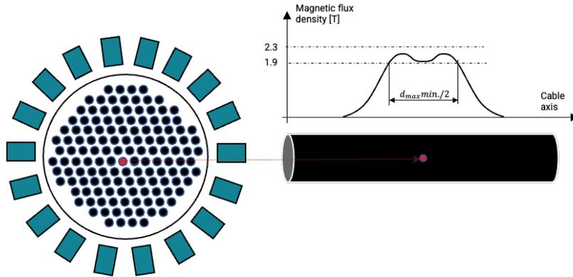
Figure 8. Cable cross-section with permanent magnet array (left), cable in axial direction with magnetic flux density plot according to DIN EN 12927-8 (DIN EN 2019).
