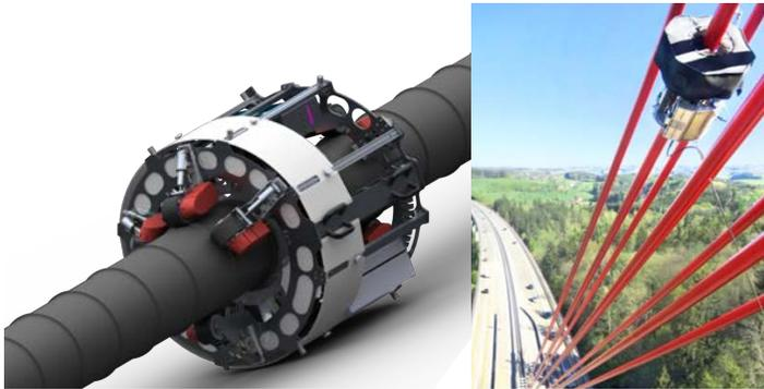
Figure 9. Inspection Bot (new generation) Size L by DYWIDAG (left), application of the Inspection Bot (first generation) Size M by DYWIDAG at Obere Argen Bridge, Germany, 2012 (right) (Kuhn 2008).
