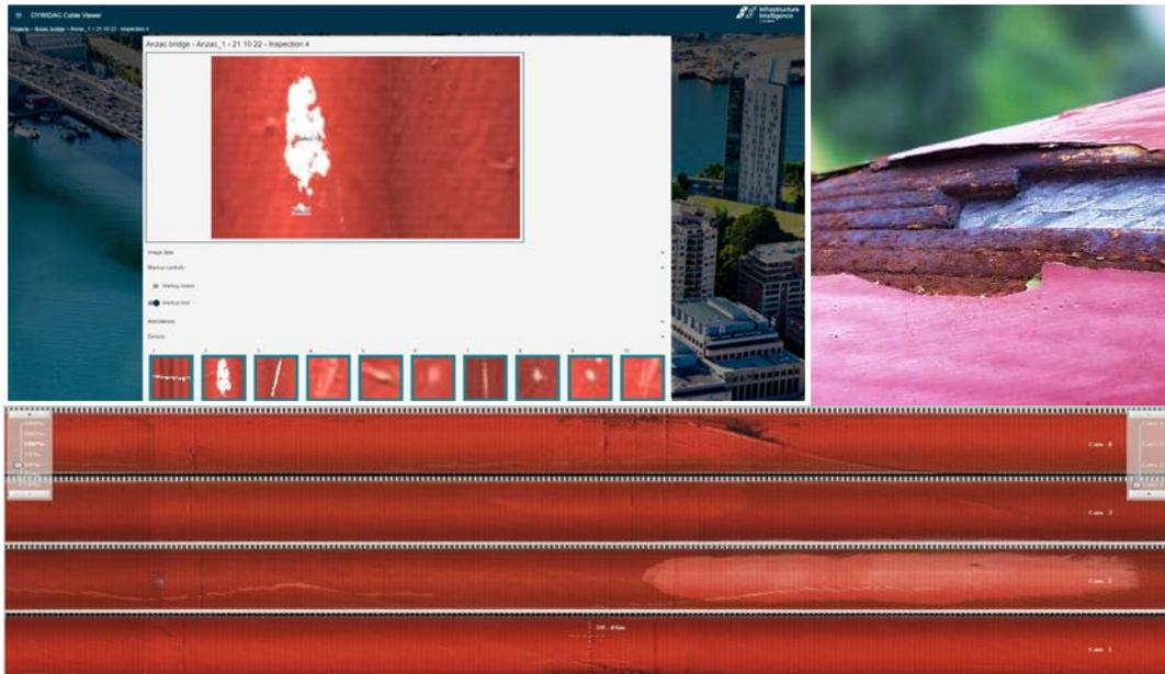
Figure 10. Visual inspection data viewer with automated defect detection by DYWIDAG.
