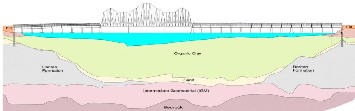
Figure 4. Generalized subsurface conditions
