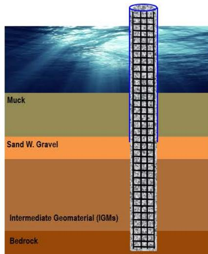
Figure 7. Drilled shaft design approach
