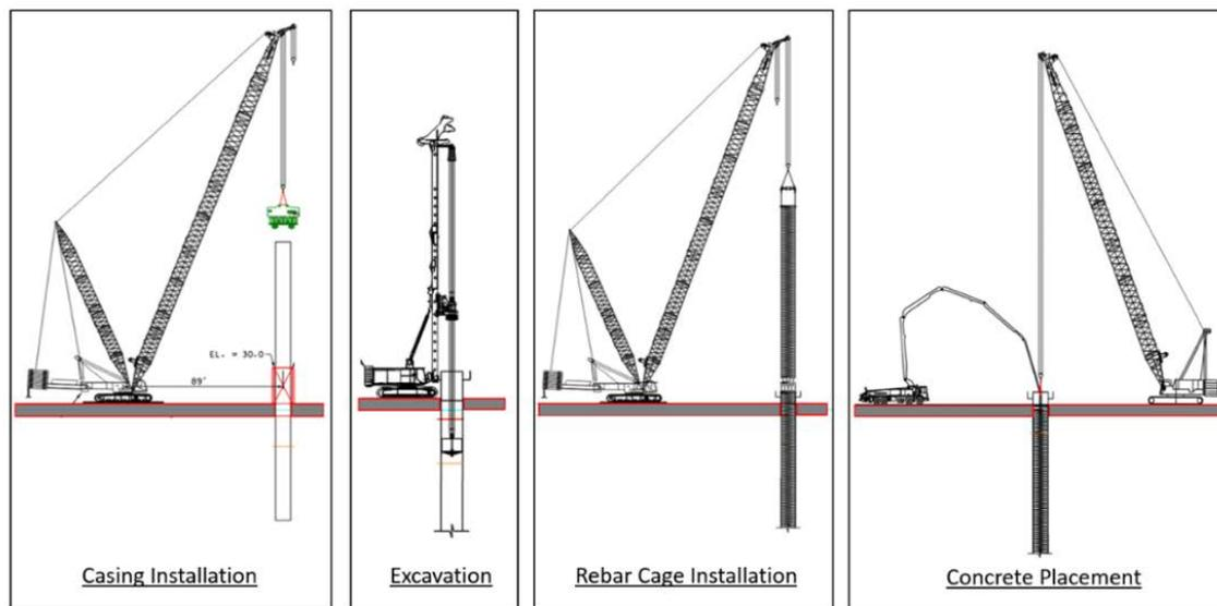
Figure 8. Test shaft construction scheme
