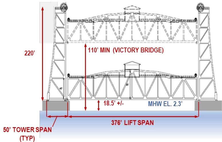
Figure 2. New replacement structure
